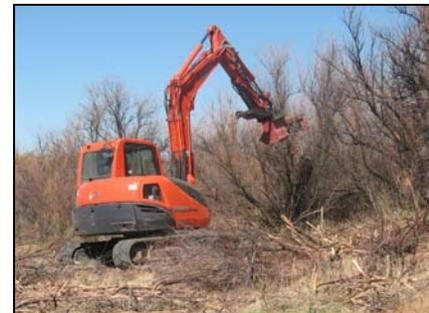
A landowner in Mack, Colorado, recently purchased an EX40 mulcher, one of the handful currently available in the United States. He runs the mulcher on a Kubota KX080 excavator. The KX08 is highly maneuverable, allowing the operator to be extremely selective in thinning operations.
